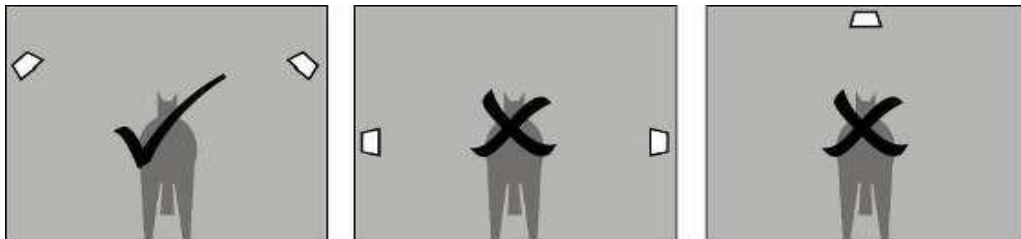
Figure 2 - Siting the BH4C infrared Heaters:
